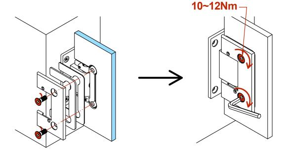
If need to install 3rd hinge for heavy door, please do not install the 3rd hinge in the center of door, the correct position should be about 8"(=20cm) under the top hinge.
