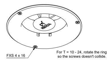
**4.** For T = 3 - 10mm, use countersunk screws and nuts (M4). First mount the ventilator from topside with 3 screws and nuts. Mount the ring from underside with 3 more screws and nuts. Make sure the screw doesn't exceed 7mm on topside.
