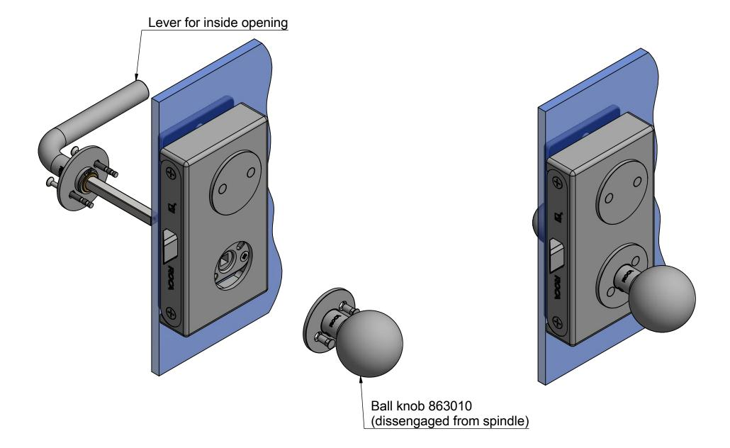
Example of configuration when use of lock case RG-461 in combination with electrical strike plate RG-589
