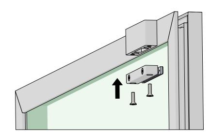
The magnetic holding force is by default ~35N. To change magnetic force adjust both screws equally; tighten the screws to reduce force and unscrew to increase.
