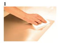
Clean surface from dust and grease with Isopropanol Std. mix ISO/Water 50/50
