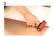
Press with the thumb or a roller. Release the liner, apply the surface area. To ensure good bond, a typical pressure should be ~100kPa
