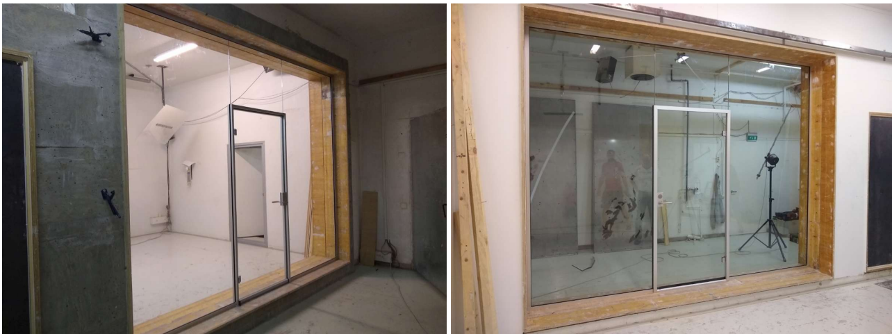
Figure A3.1. Specimen as seen from the source room (left) and the receiving room (right).
