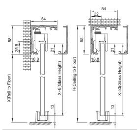
Standard Rail Length 2000mm CW MAX. = 950mm (Option Rail Length 2400mm, CW MAX. = 1150mm) CW = Clear opening width Glass Door Width = CW+60 Rail Length = (2 X CW)+100 Entry Width = CW
